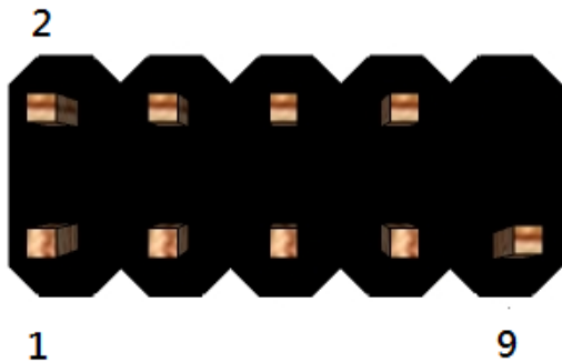
Figure 8: RS232 COM Port Header (2D)▲
